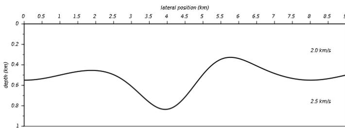
Figure 1: Simple model representing a reflector between two layers with propagation velocity of 2.0 km/s above and 2.5 km/s below it.
