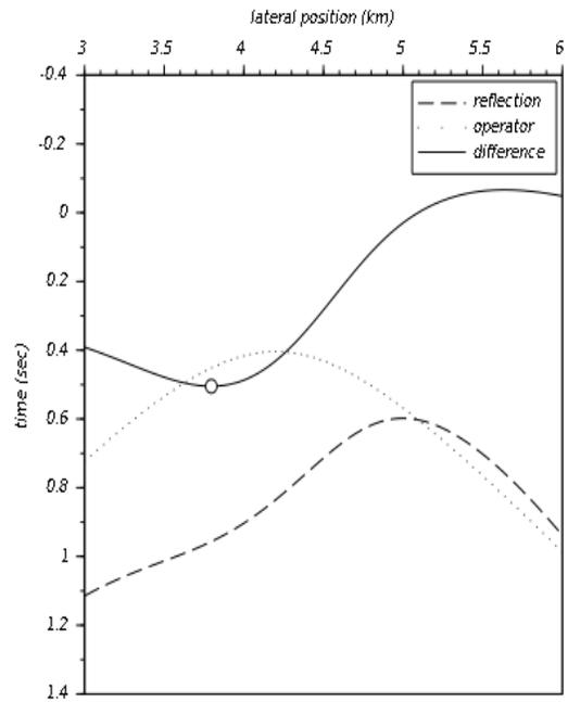
Figure 3: Reflection traveltime curve for a source at 4.5 km, operator traveltime for a focal point at 4.2 km and the difference between them. The stationary point (circle) indicates the traveltime from the source to a virtual receiver at the focal point.
