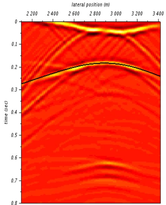
Figure 7: Superposition of the optimised operator over the CFP gather for a focal point positioned at 2700 m.
