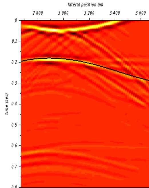
Figure 8: Superposition of the optimised operator over the CFP gather for a focal point positioned at 3300 m.
