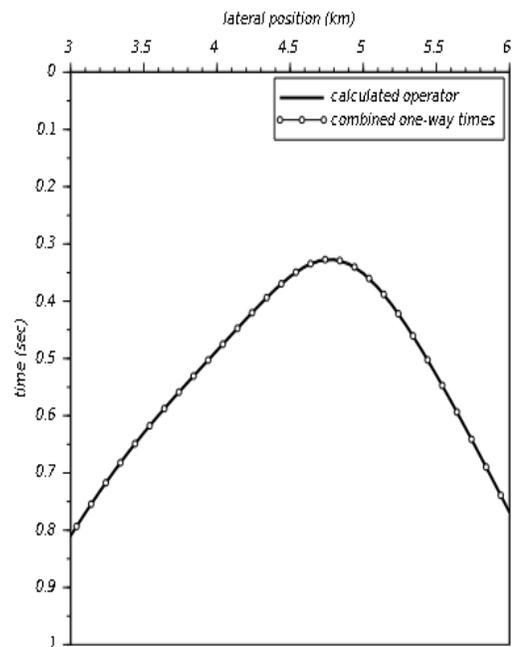
Figure 2: Superposition of the combination of all one-way traveltimes over the calculated operator.
