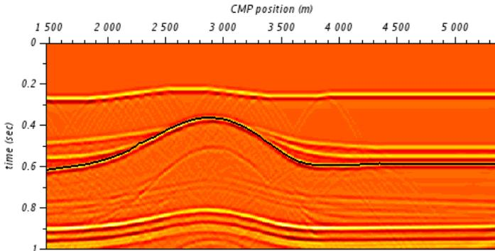
Figure 4: Reflection traveltime curve extracted from the common offset section (black line) for an offset of -60 m.
