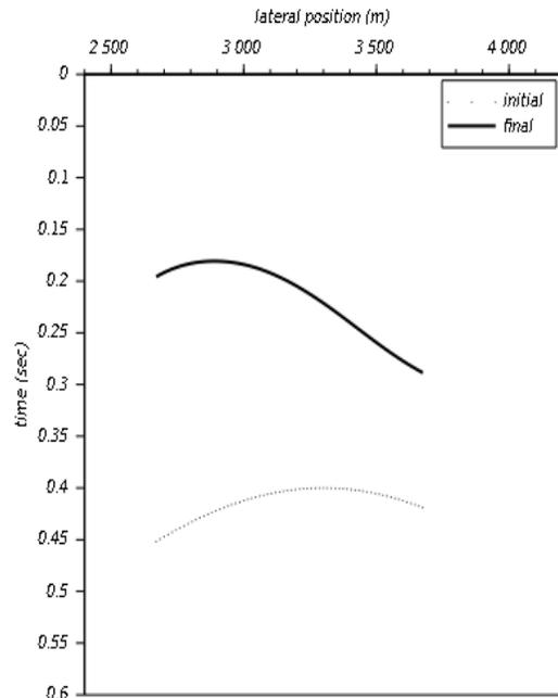
Figure 5: Optimisation of the initial operator at 3300 m. The dotted and solid lines express the inital and optimised operators, repectively.
